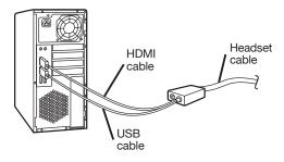
**Note:** To minimize cable thickness, each DK2 cable is individually calibrated for maximum HDMI signal integrity over the length of the cable. As such, joining multiple HDMI cables via passive couplers is not recommended for use with the DK2 cable as the additional length is not compatible with this calibration.
